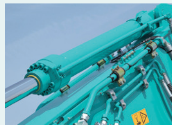
Reinforced bucket cylinder Use of a dedicated cylinder with reinforced components such as the head cap.
