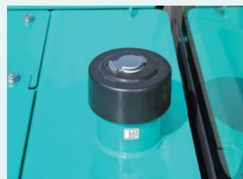
Dust-proof fuel tank cap The fuel cap is lined with rubber so that dust does not easily contaminate the fuel tank.
