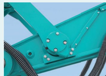
Bucket angle sensor cover The cover protects the bucket angle sensor installed on the idler link. A cable guard also protects the electrical cables from being cut off.
