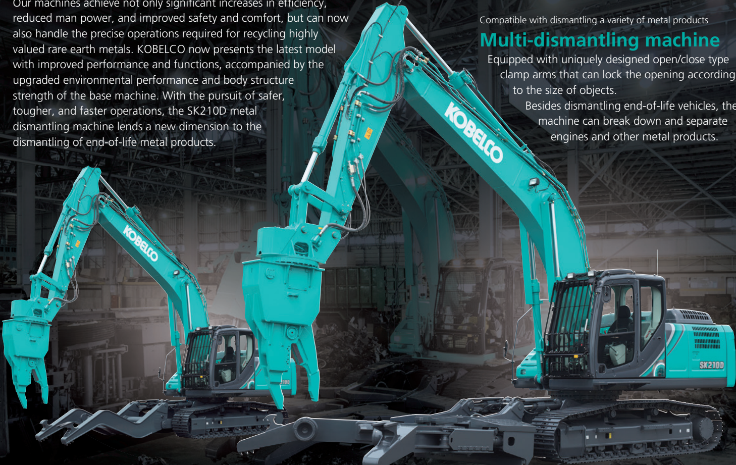
Specialized machine for dismantling end-of-life vehicles
