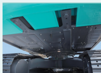
Upper main body undercover The 6 mm thick reinforced cover protects the inner devices.
