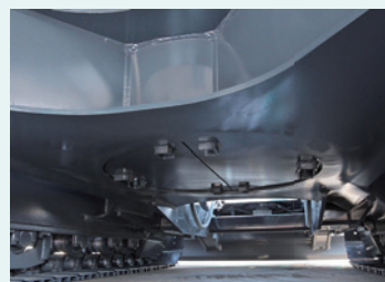
Lower undercover The lower car body structure is fitted underneath with a 9 mm thick reinforced cover.
